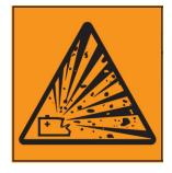
THE LEAD ACID BATTERIES MAY GENERATE EXPLOSIVE HYDROGEN GAS DURING NORMAL OPERATION. KEEP SPARKS, OPEN FLAMES, OR LIT TOBACCO AWAY FROM THE BATTERIES. DURING BATTERY CHARGING, PROVIDE FOR ADEQUATE VENTILATION IN THE AREA. DO NOT CHARGE A FROZEN BATTERY. CAREFULLY STUDY THE PRECAUTIONS SPECIFIED BY THE BATTERY MANUFACTURER RELATIVE TO THE SPEED OF CHARGING RECOMMENDED AS WELL AS THE POSSIBILITY OF REMOVAL OF THE CELL CAPS DURING CHARGING.
