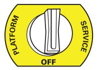
To turn the personnel lifter off, turn the selector switch to "OFF".
