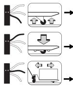
To raise the load, push down on the fingertip control. Pump the handle to raise the load from the floor.
