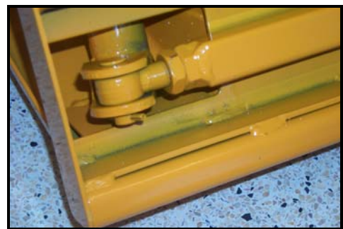
Photo 2 – tightened jam nut against welded nut
