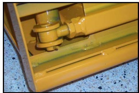
Photo 2 – tightened jam nut against welded nut
