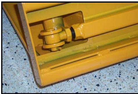
Photo 1 – jam nut loose
