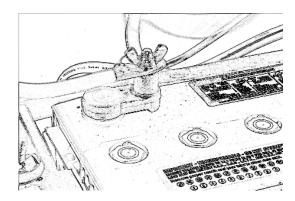
both wires to the negative battery post and tighten the butterfly nut.
