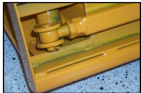
Photo 2 – tightened jam nut against welded nut
