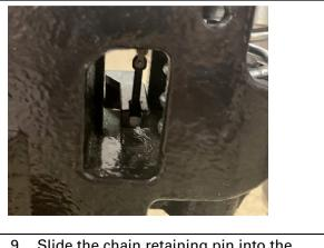
9. Slide the chain retaining pin into the retaining clip inside the pump housing.
