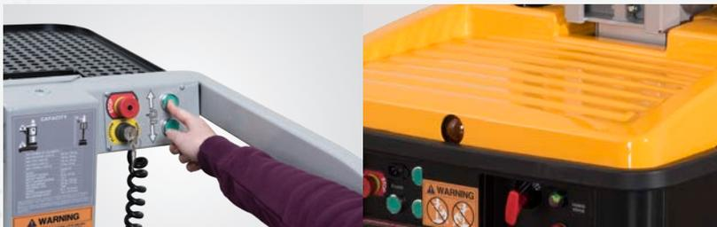
Operator compartment allows easy access to the key switch and lift/lower controls
