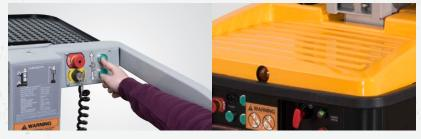
Operator compartment allows easy access to the key switch and lift/lower controls
